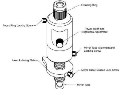
peaks and valleys of the threads as the mirror tube rotates through the threads. The brightness of the LED is controlled with the rotation of the power on/off switch.
